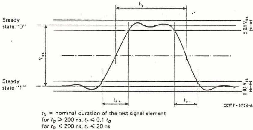
FIGURE 4/V.11 - Generator dynamic balance and rise time measurement
