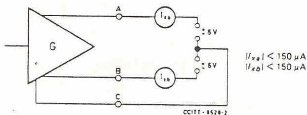
FIGURE 12/V.11 Generator output leakage current measurement
