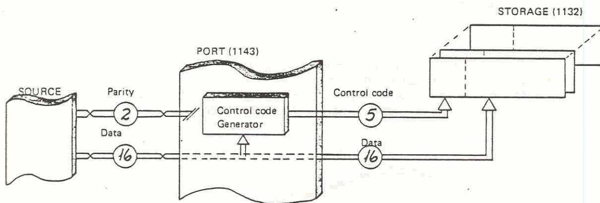
Figure 1.16: Data Flow on Write
