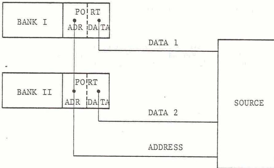
Figure 2.4: Two 16 Bit Banks Accessed as One 32 Bit Bank
