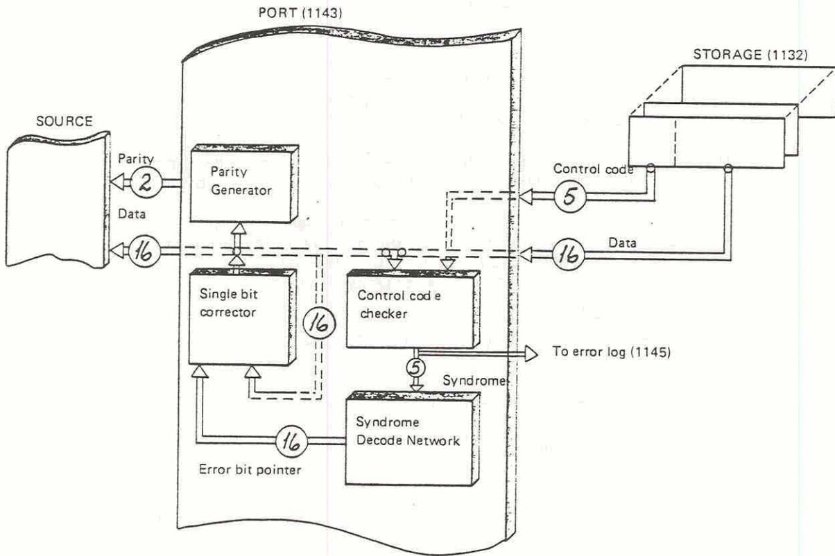
Figure 1.18: Reading Data (Single Error)
