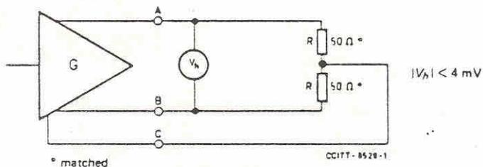
FIGURE 11/V.11 High impedance state static measurement
