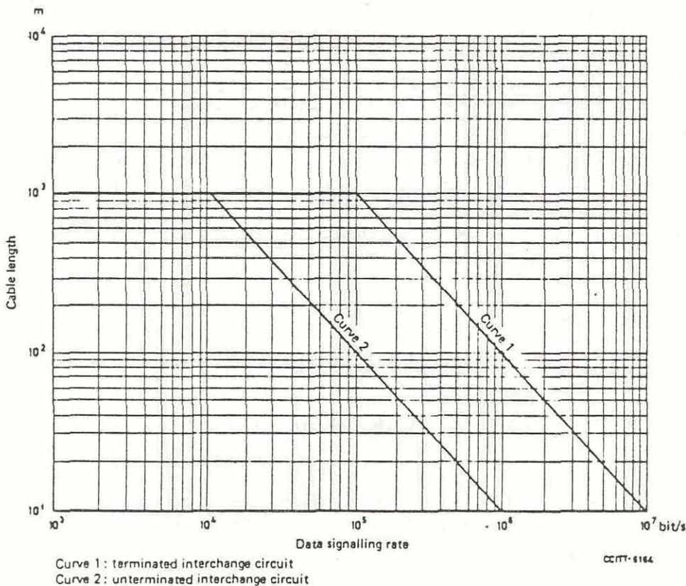
FIGURE 8/V.11 - Data signalling rate vs cable length for balanced interchange circuit
