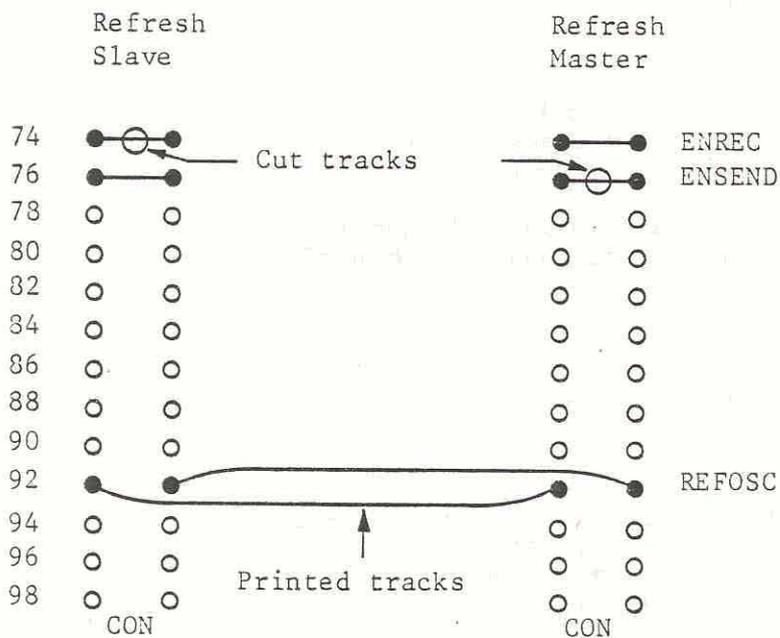
Figure 5.5: Refresh Synchronization at Control Modules in Slot 9 or 28.
