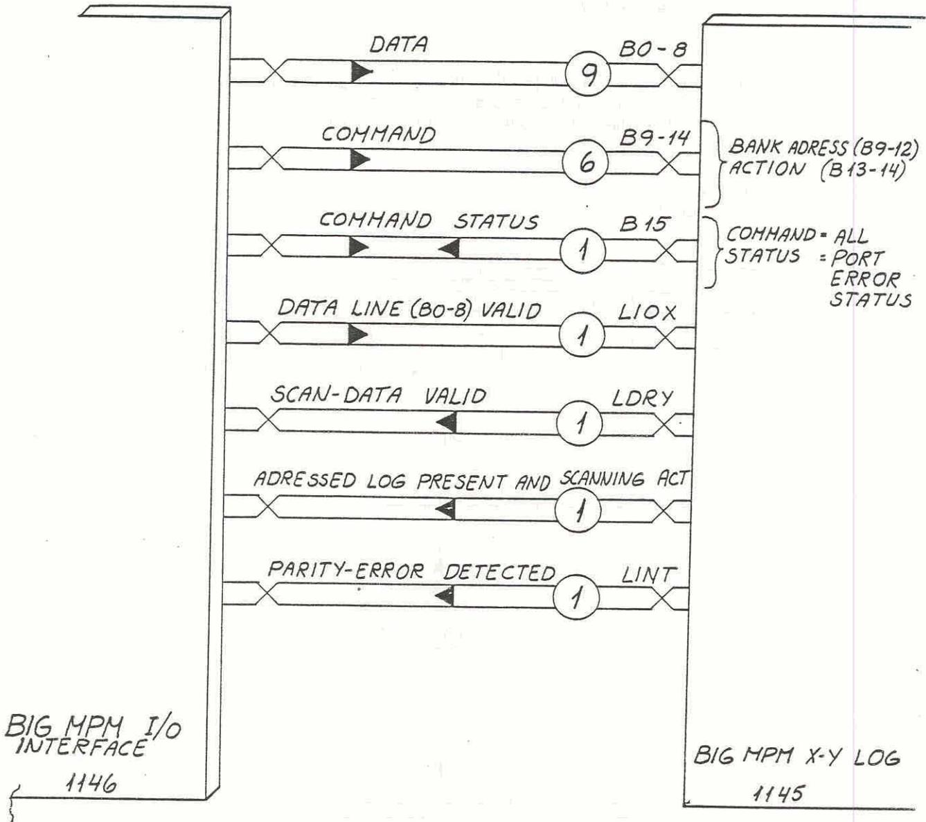
Figure 3.2: I/O Module to Error Log Module Communication
