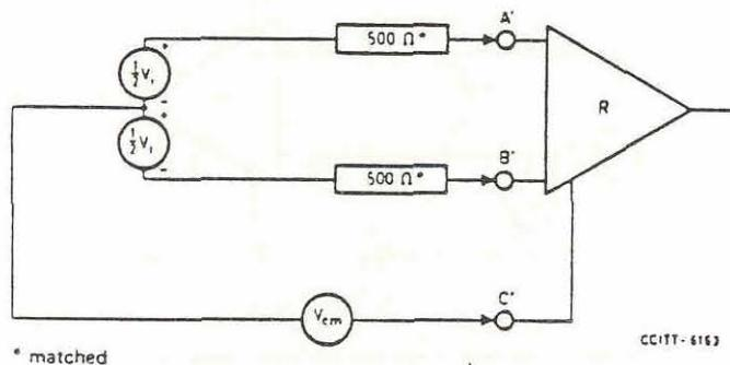
FIGURE 7/V.11 -- Receiver input balance test
