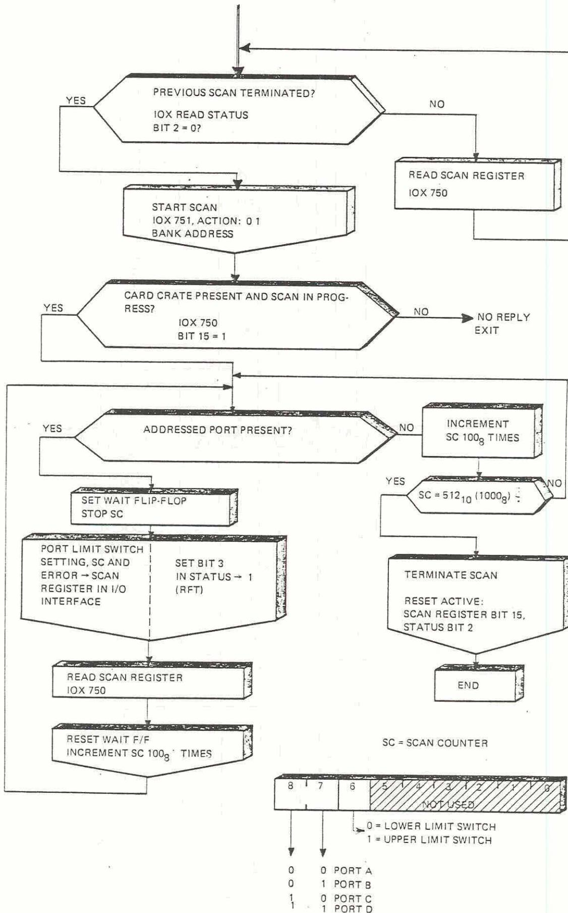
Figure 3.7: Action: 01 Scan of Port Status — Flow Diagram
