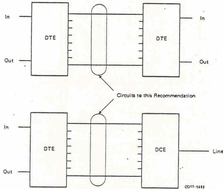
FIGURE 1/V.11 - Typical applications of balanced interchange circuits
