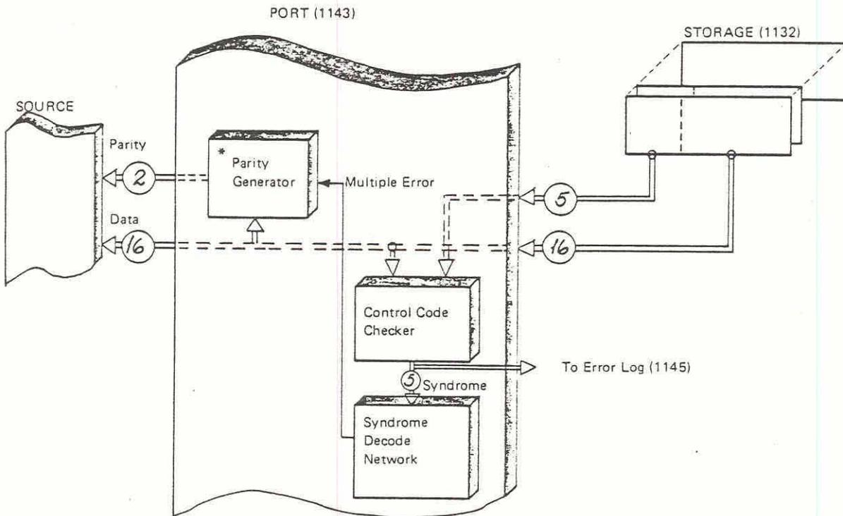
\* when multiple error is detected parity bit for lower byte is forced false (BDL 16)
