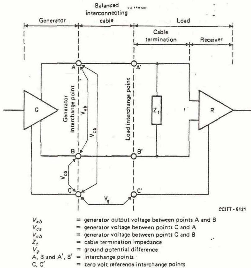
FIGURE 2/V.11 – Symbolic representation of a balanced interchange circuit
