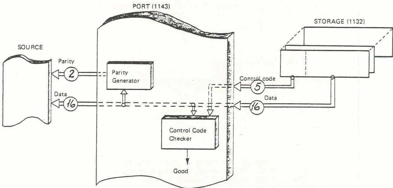
Figure 1.17: Reading Data (No Error)
