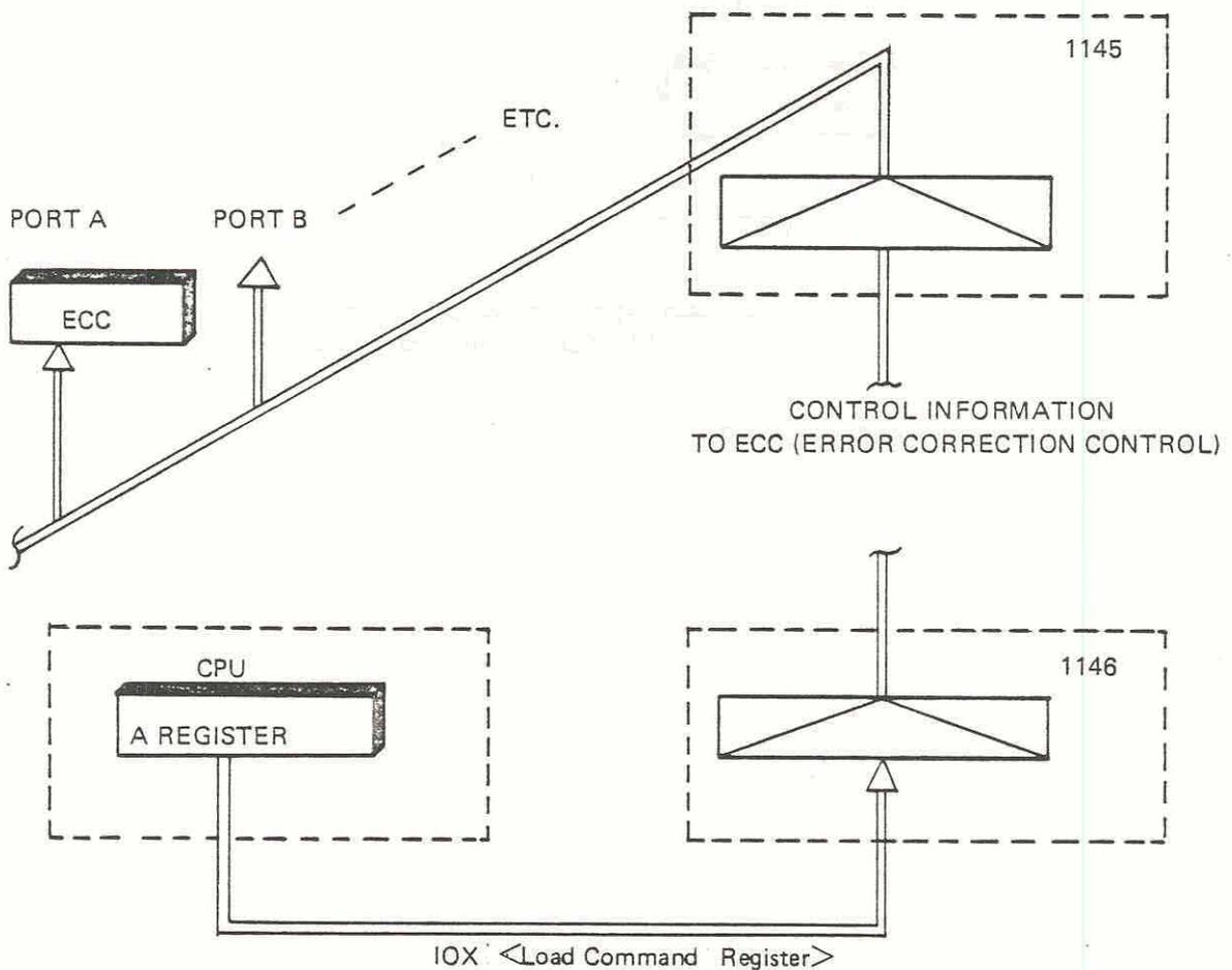
Figure 1.7: Write ECC Register
