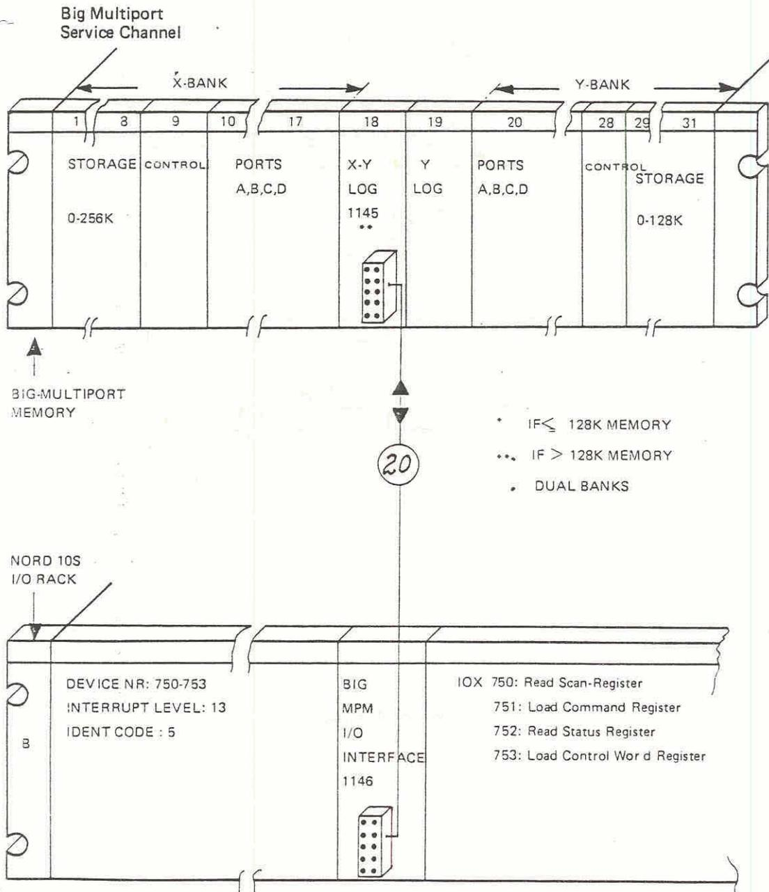
Figure 3.1: BPPM Service Channel
