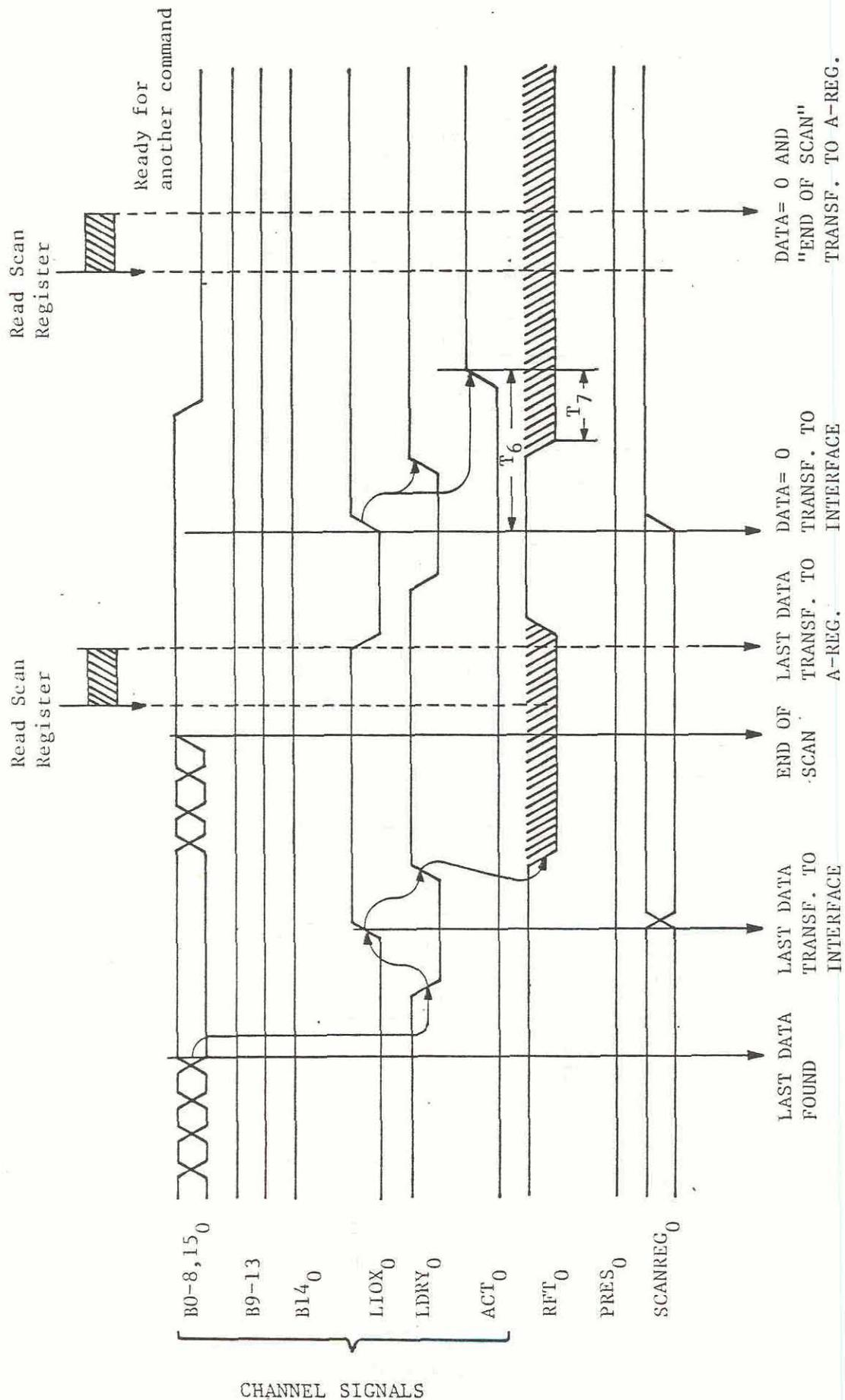
Figure 3.10: Termination of a Scan
