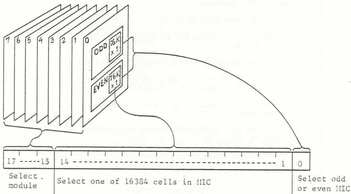
Figure 1.3: Use of Internal Bank Address
