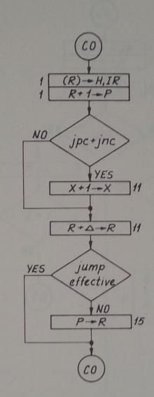
NOTE: t12 - 15 is "inserted" only if jump not effective and does not exist with jump effective. Controlled by signal NEXT to time counter.
