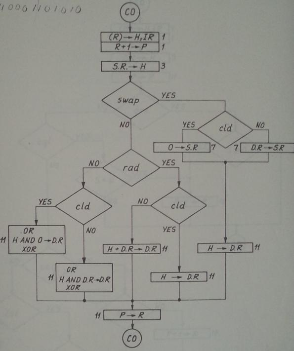
If D.R.=P  $P \rightarrow R$  is replaced by  $S \rightarrow R$ . If IR7=1 H is replaced by one's complement of H in the diagram above.
