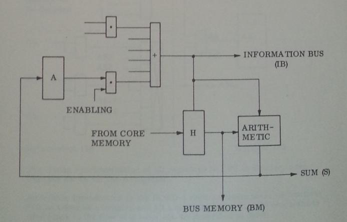
One register is enabled at a time and presented at the IB terminals, and as input to the arithmetic. Data from memory goes via the H-register and the BM input to the arithmetic. For inter-register operations one of the operands (source) is first transferred to the H-register before IB is switched to the other operand. The output of the arithmetic is then routed back to all registers where it may be strobed into register flip-flops.
