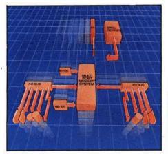
controllers can be connected directly to the memory system and thereby utilize the full bandwidth. Even though the operating system is virtual, the memory system is designed to handle up to 2000 MB of real memory.
