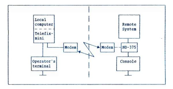
Figure 1. Telefix-mini installation.
