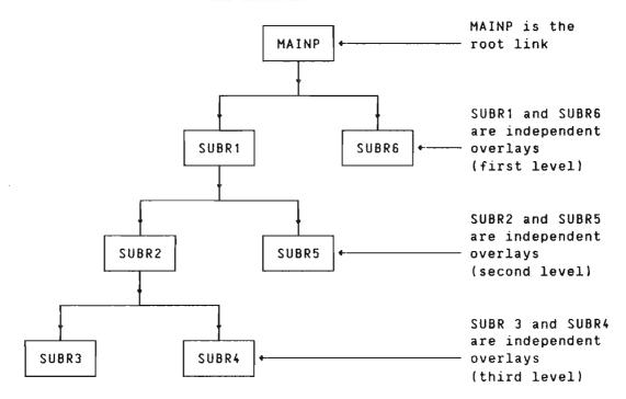
SUBR4 depends on SUBR1 and SUBR2 so they must be in memory when in order to execute SUBR4. The chain of links which a link depends on is referred to as the **path** of the link. The action of bringing a link into memory is termed **path loading** and the chain of links branching away from a link is known as the **extended path** of that link. In the previous example, the path of SUBR4 is MAINP, SUBR1, and SUBR2. There are three extended paths of SUBR1:
