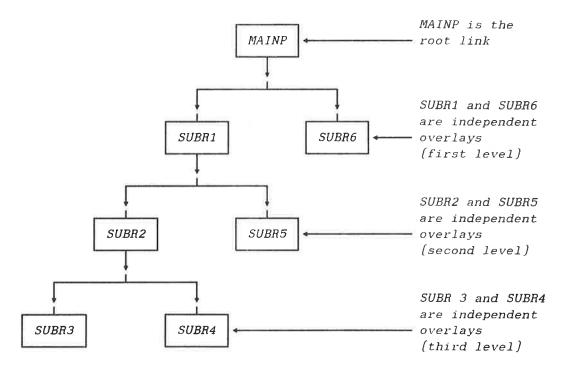
SUBR4 depends on SUBR1 and SUBR2 so they must be in memory when in order to execute SUBR4. The chain of links which a link depends on is referred to as the *path* of the link. The action of bringing a link into memory is termed *path loading* and the chain of links branching away from a link is known as the *extended path* of that link. In the previous example, the path of SUBR4 is MAINP, SUBR1, and SUBR2. There are three extended paths of SUBR1: The Overlay System The Multilevel Overlay System
