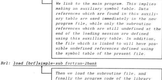
finally the program code of the library routines, plus the data referenced by library routines which have not been referenced in the main program. In this way, some code is duplicated, reducing segment switching time.
