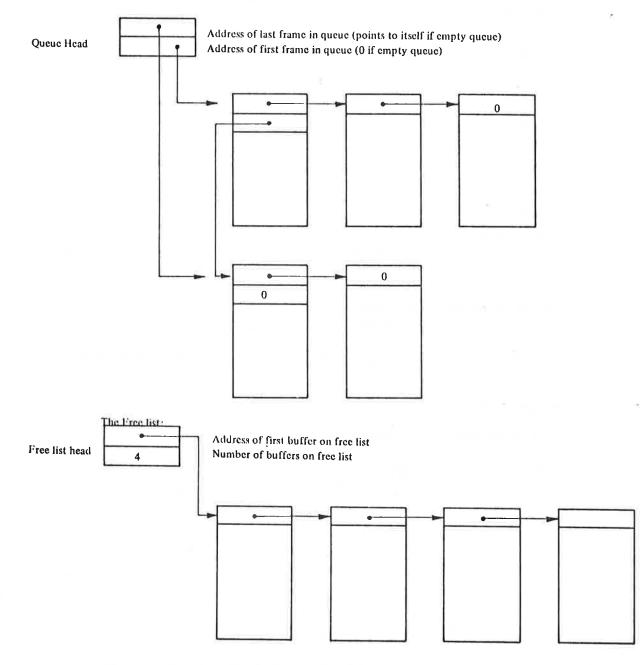
The size of each buffer is  $34_{\scriptscriptstyle B}$  words, giving a maximum of 5 buffers for one frame.
