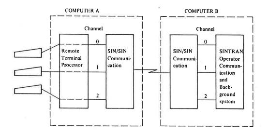
The main task of the Remote Terminal Processor in computer A is to copy the input given from the terminal to a communication channel, and to copy the output returned on the channel to the terminal.
