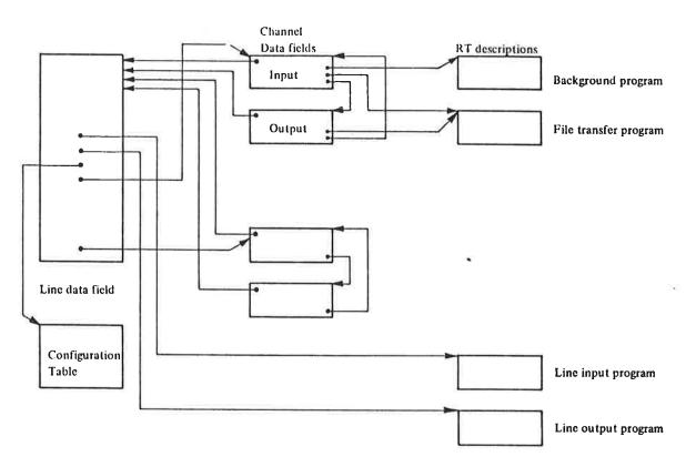
The internal data fields for a communication line is illustrated below:
