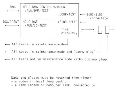
a remote CPU with HDLC echoing the signals.
