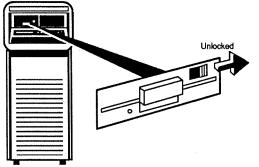
1. If the locking switch is in locked position (red mark showing), push it rightwards to unlocked position.
