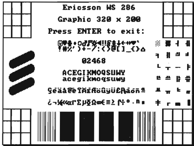
Fig 7.25: PC Diagnostic - graphic 320x200 display test
