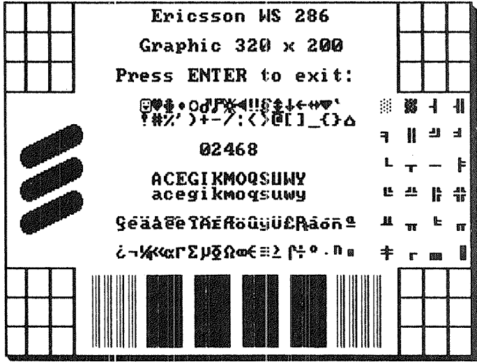
Fig 7.25: PC Diagnostic - graphic 320x200 display test
