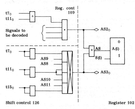
The timing synchronization of all registers in CPU is similar to the example shown for the A-register.
