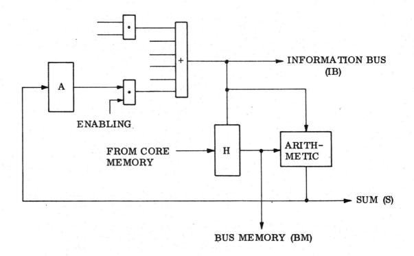
One register is enabled at a time and presented at the IB terminals, and as input to the arithmetic. Data from memory goes via the H-register and the BM input to the arithmetic. For inter-register operations one of the operands (source) is first transferred to the H-register before IB is switched to the other operand. The output of the arithmetic is then routed back to all registers where it may be strobed into register flip-flops.
