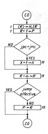
NOTE: t12 - 15 is "inserted" only if jump not effective and does not exist with jump effective. Controlled by signal <u>NEXT</u> to time counter.
